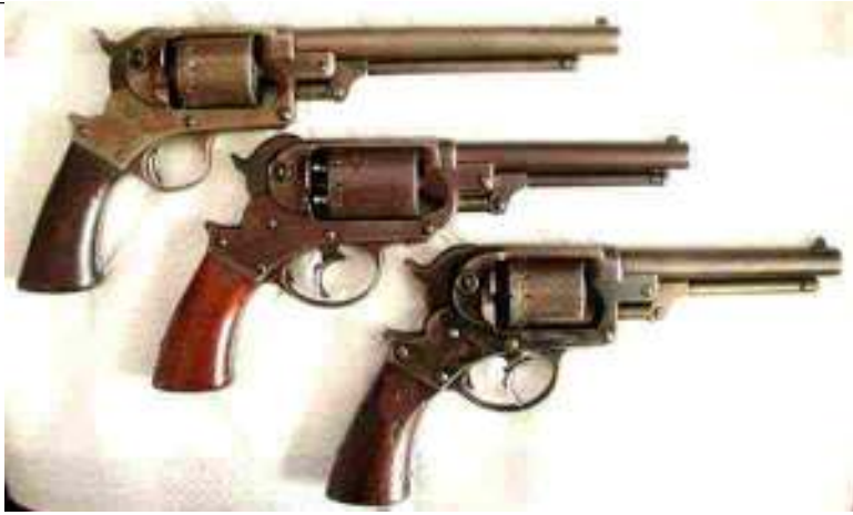
Starr 1863 Single Action .44 caliber Army, 1858 Double Action .36 caliber Navy, and 1858 Double Action .44 Army revolvers Specifications: Single-action: Length: 13.75" Weight: 3 lbs. Caliber: .44 Double-action: Length: 11.625" Weight: 2 lbs., 12 oz. Caliber: .44
