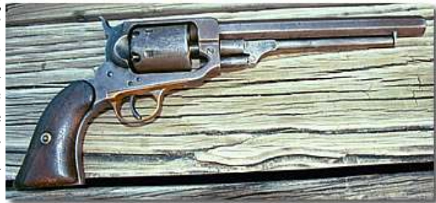
Whitney "Navy" revolver Specifications: Length: 13.125" Weight: 2 lbs., 7 oz. Caliber: .36
