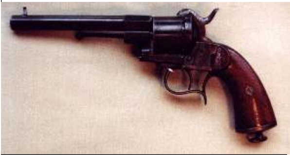
Lefauchaux Revolver Specifications: Length: 11.5" Weight: 2 lbs., 6 oz. Caliber: 12 mm (.44)
