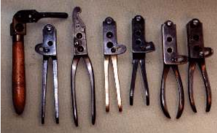
Bullet Molds for various Civil War revolvers From left to right: Starr Savage Tranter Massachusetts Arms Manhattan Allen & Wheelock Colt
