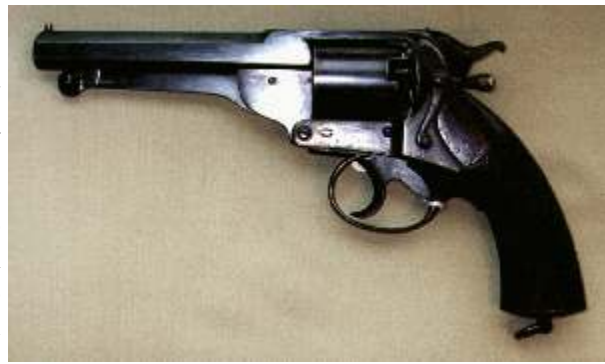
Kerr Revolver Specifications: Length: 10.8" Weight: about 2.5 lbs. Caliber: .44
