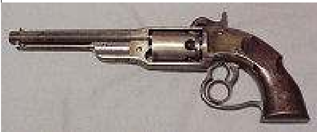
Savage Navy Revolver Specifications: Length 14.25” Weight: 3 lbs., 7 oz. Caliber: .36
