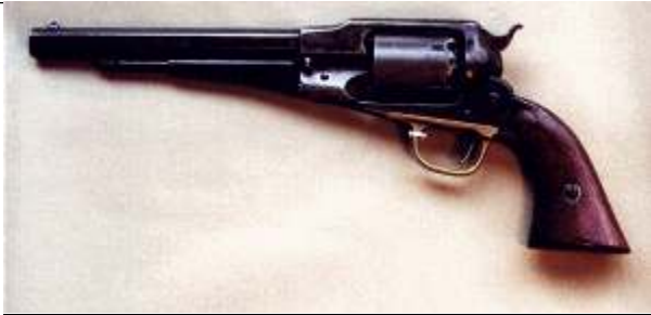
Remington Model 1861 Army Revolver Specifications: Length 13.75 Weight: 2 lbs., 14 oz. Caliber: .44
