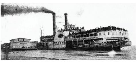
Cahaba Prison camps, were brought to the *Sultana*, a mechanic was brought down to work on the leaky boiler. Although the mechanic wanted to cut out and replace a ruptured seam, the ship's Captain knew that such a job would take a few days and cost him his precious load of prisoners, rather only a temporary repair was made to the boiler.
